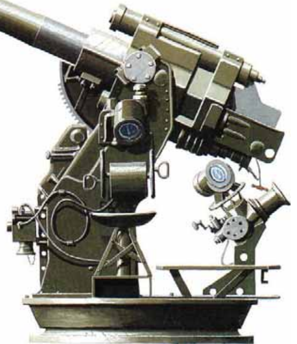
Above: In 1941 the American 3-in (76.2-mm) gun was still in service in several forms. This static version was the 3-in Gun M4 on Mount M3, and was used in such locations as the Philippines and the Canal Zone.
