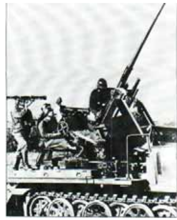
First produced in 1937, the SdKfz 6 AA variant mounted a 3.7-cm (1.456-in) Flak 36 on an open platform. The presence of a crew member with range finder dates the picture as early in the war; later they were withdrawn to save manpower.
