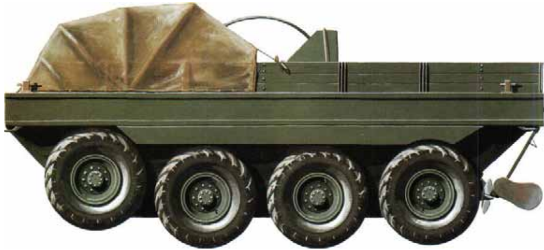
The Terrapin was powered by two Ford V-8 petrol engines and was driven in the water by two propellers at the rear. There were two cargo holds and the driver sat in the centre of the vehicle.
