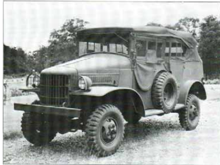
The Dodge T215 WC23 was a 1/2-ton command and reconnaissance vehicle of the same family as the T207. The 1941 pattern vehicles are identifiable from the heavier 1942 models by their sloping bonnet.
