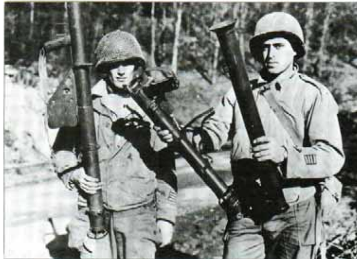
The original M1 bazooka is shown on the left and the M9 on the right. The M1 could be broken down into two halves, which greatly assisted carrying and stowage inside vehicles. By the time the war ended a version of the M9 was being produced in aluminium for lightness; this was the M18.
