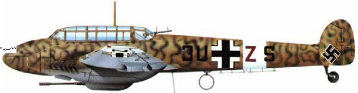
A Messerschmitt Bf 110E of 8./ZG 26 based at Berca, North Africa, in September 1942. It is armed with the powerful MK 101 30-mm cannon, for use in the tank-busting role.
