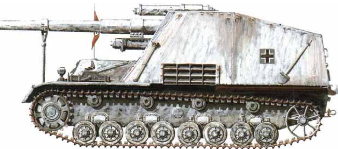
Above: The Hummel (bumble bee) was a purpose-built German vehicle that used components from both the PzKpfw III and IV. Used on all fronts, it was a successful weapon that remained in production until the war ended. It had a crew of five.
