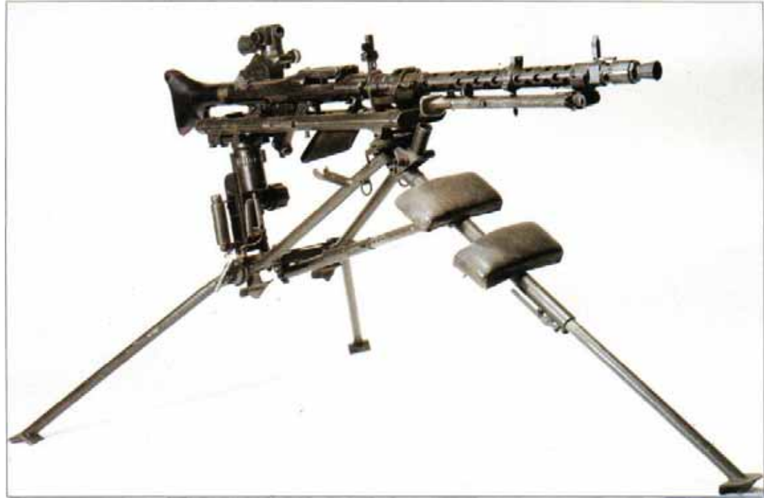
An MG 34 mounted for the heavy machine-gun role on a Lafette 34 tripod and complete with the indirect-fire sight; the pads on the front leg rested against the carrier's back when folded for transport.
