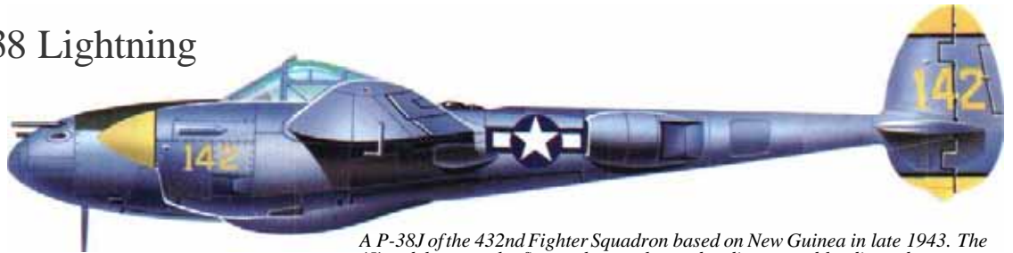
A P-38J of the 432nd Fighter Squadron based on New Guinea in late 1943. The 'J' models were the first to have relocated radiators and leading-edge tankage.
