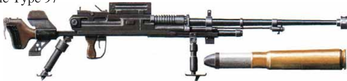
The Japanese Type 97 anti-tank rifle was a heavy weapon that weighed 51.75 kg in action, mainly due to the gas-operated semi-automatic mechanism. It had a calibre of 20 mm (0.787 in) and required a crew of two men to fire and four to carry it, using a system of frames.
