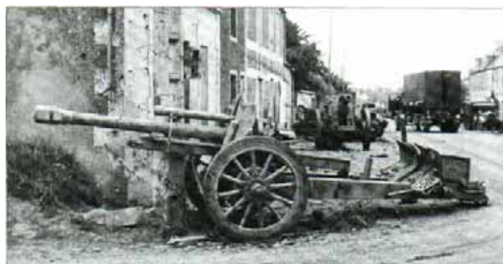
Above: Abandoned 10.5-cm leFH 18(M) howitzers in Normandy in June 1944. Note the obvious bulk and weight of the trail legs and spades that combined to make this howitzer too heavy for the mobile field role.
