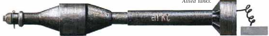
The German RP43 was inspired by the American bazooka, but used a larger 8.8-cm (3.46-in) rocket. Sometimes known as Panzerschreck , this weapon had a range of 150 m (165 yards) and could knockout all Allied tanks.
