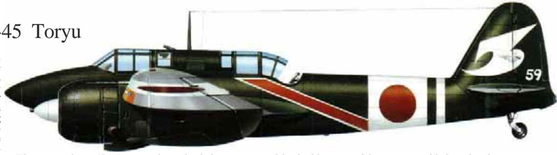
The Kawasaki Ki-45 KA1c was the night-fighter variant of this highly successful twin-engine fighter-bomber. Carrying one forward-firing and two obliquely-mounted upward-firing cannon, this is a machine belonging to the 1st Chuutai, 53rd Sentai, based at Matsudo in early 1945.
