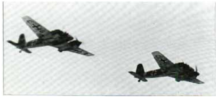
The Henschel Hs 129 was designed to a 1937 specification for an armoured, twin-engined ground attack aircraft. Far superior to Allied equivalents, it showed how much importance the Germans attached to close air support.
