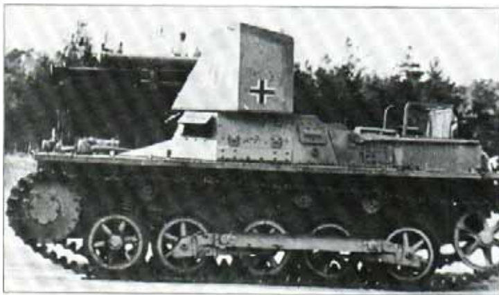
This photograph of a Panzerjäger I shows the extemporized nature of this early German conversion, made in an attempt to prolong the service
