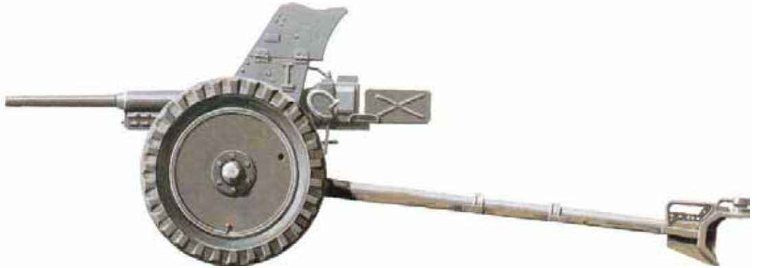
Above: The original 3.7-cm Pak 35/36 produced during the late 1920s had spoked wheels for horse traction, but by the mid-1930s these had been replaced by steel disc wheels for motor traction. It was a light and low gun that was at first issued to all arms of the Wehrmacht.
