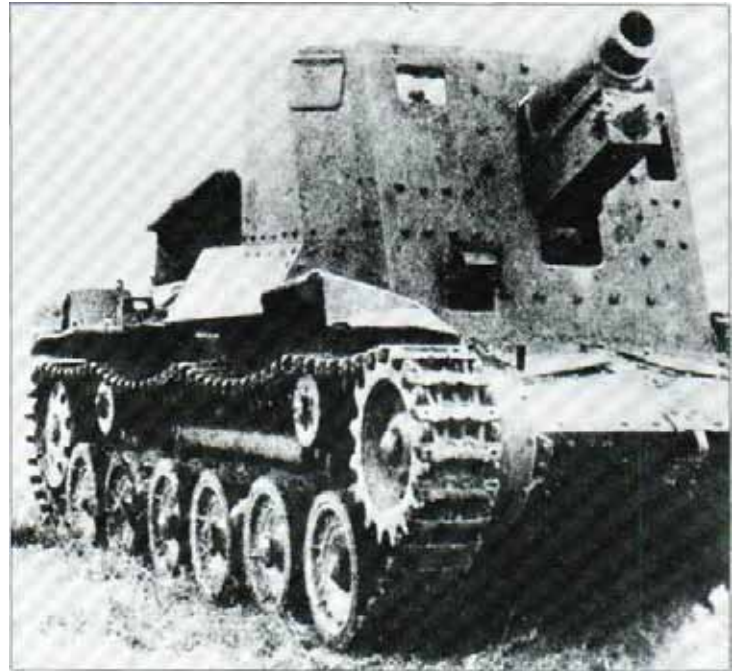
The Type 97 had its 150-mm howitzer mounted in place of the turret normally carried. The howitzer was
