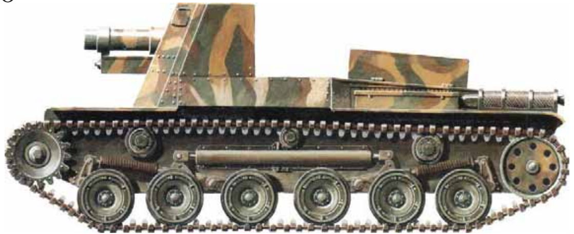
Above: The Type 97 mounted a short Type 38 howitzer with limited range, but the Japanese were never able to produce the numbers required and they were mainly used in ones and twos as local fire-support weapons.
