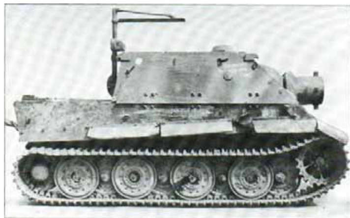
Above; This side shot of a Sturmtiger shows the large armoured superstructure, mounting the 38-cm (14.96-in) rocket projector with the roof-mounted crane needed to load the projectiles in to the interior through a hatch at the rear.
