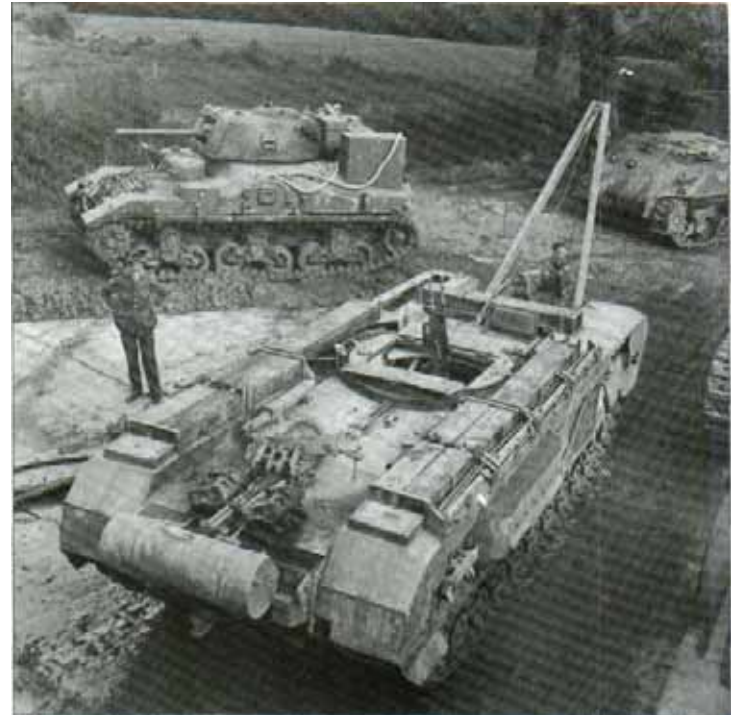
A Churchill ARV (Armoured Recovery Vehicle) MkI has its front jib erected and twin 7.7-mm (0.303-in) Bren machine-guns mounted in the hull. This vehicle had a crew of three and carried special tools and welding equipment for the recovery role. The vehicle was basically a turretless Churchill MkIV.
