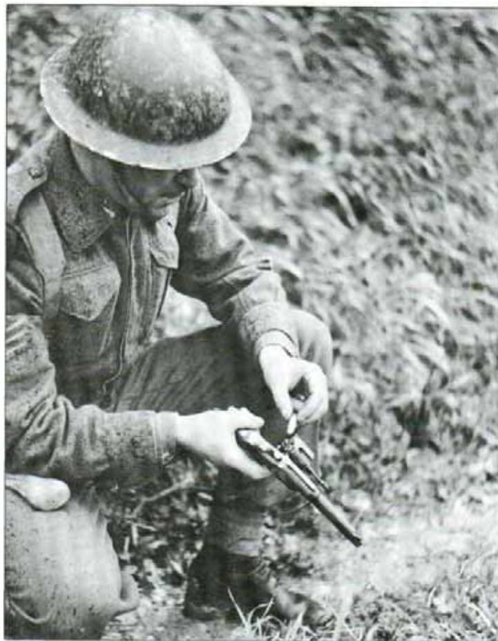
Above: A Canadian sergeant loads a Smith & Wesson 0.38/200 revolver. Empty cartridge cases were ejected by moving out the cylinder to the left and pressing a plunger normally under the barrel.
