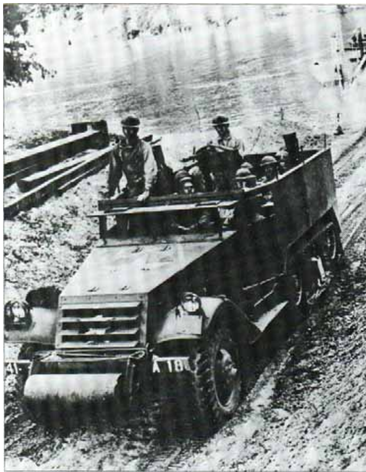
An early shot of the M2 halftrack, taken when the US Army was still using the World War I helmets and equipment. This vehicle still has the original centre-mounted machine-
