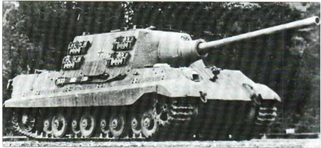
Above: Two types of suspension were used on the Jagdtiger. This example has the Henschel suspension; the other type used larger road wheels from Porsche. Based on the Tiger II tank chassis, only about 70 were produced, and it was the heaviest AFV to see service during World War II.
