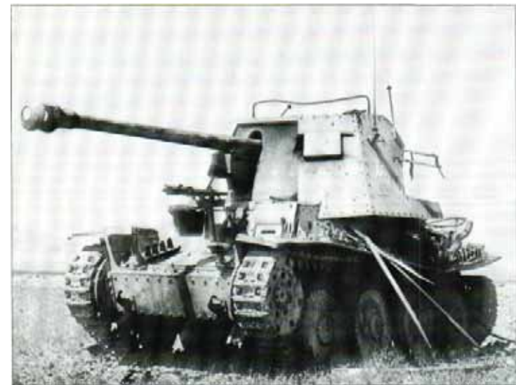
The later Marder IIIs had their main gun position moved to the rear of the chassis and the engine to the front. This provided a better-balanced and
