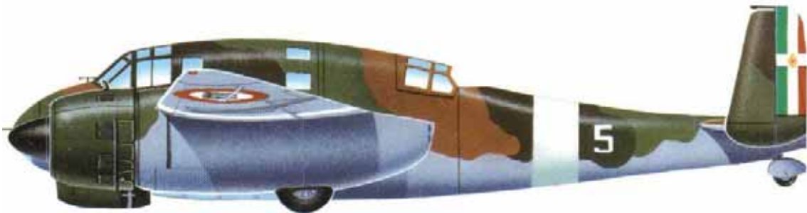
Above: Formerly of CBA 1/51 of the Armée de l'Air, this Breguet Bre. 693 is pictured after being transferred to the Regia Aeronautica in 1943. The red of the French roundels were retained, with the Italian fasces replacing the blue.
