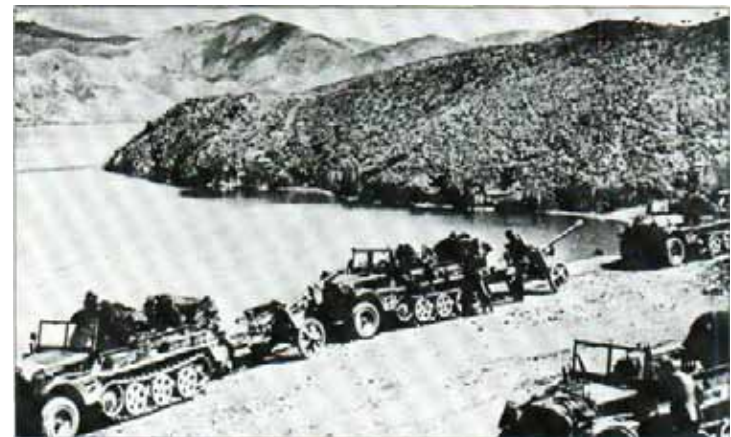
SdKfz 10 leichter Zugkraftwagen It tractors are being used here in their intended role to tow 5-cm (1.97-in) Pak 38 anti-tank guns. The vehicles
