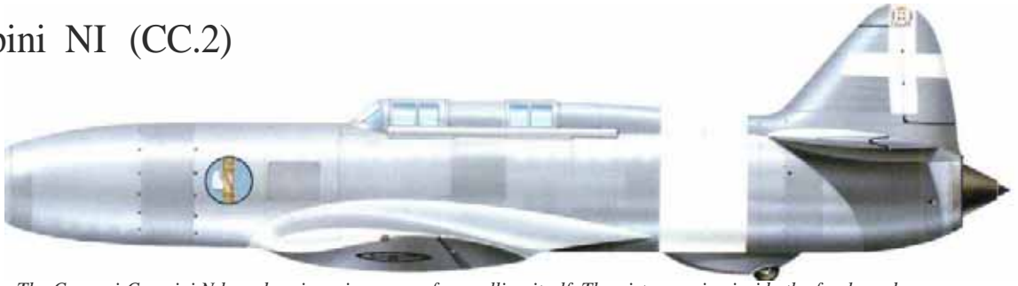
The Caproni-Campini NI used an ingenious way of propelling itself. The piston engine inside the fuselage drove a ducted fan and fuel was bled and ignited in the compressed air emitted through the tailpipe.
