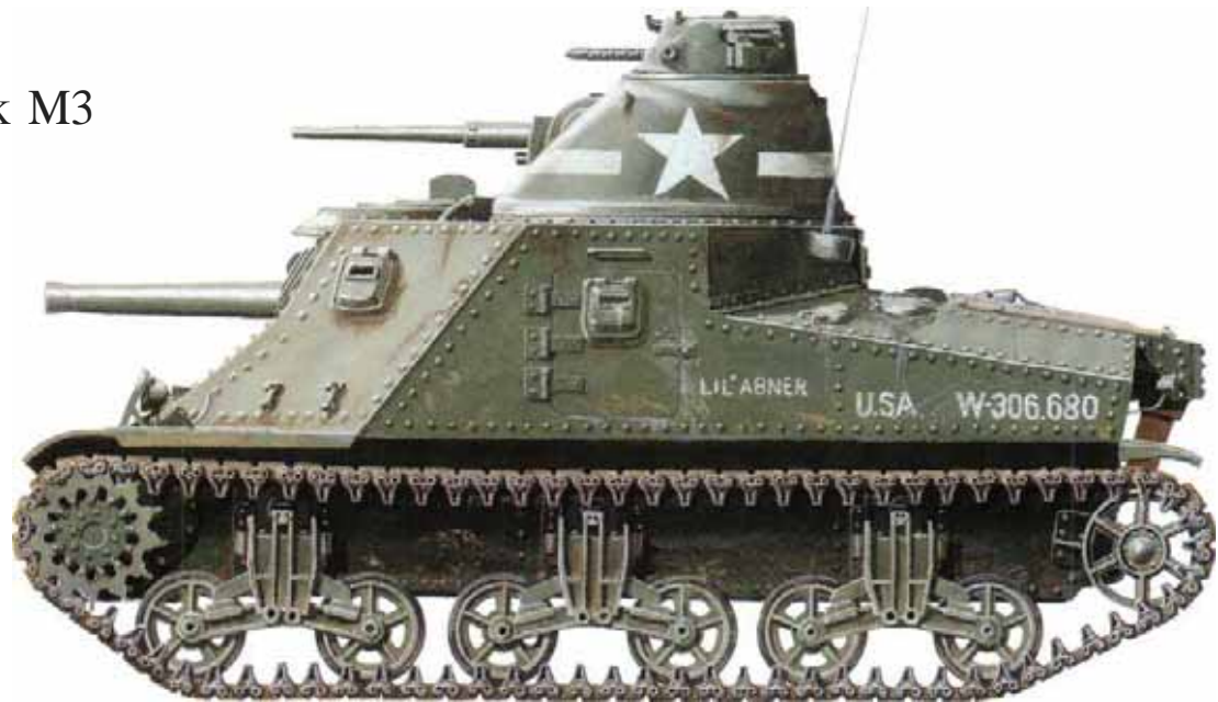
Above: The M3 General Lee tank was a hasty design, but it had a powerful 75-mm gun which gave Allied tanks a parity with German tanks for the first time.
