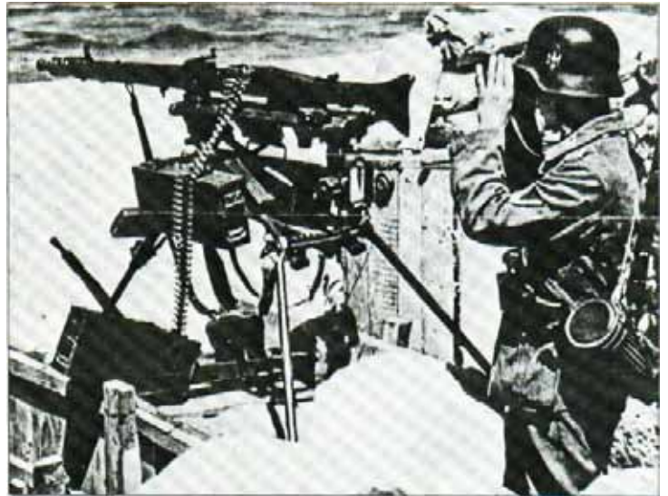
Above: An MG 42 mounted on the Lafette 42 for the heavy machine-gun role; this heavy tripod could be quickly adapted for the anti-aircraft fire role.
