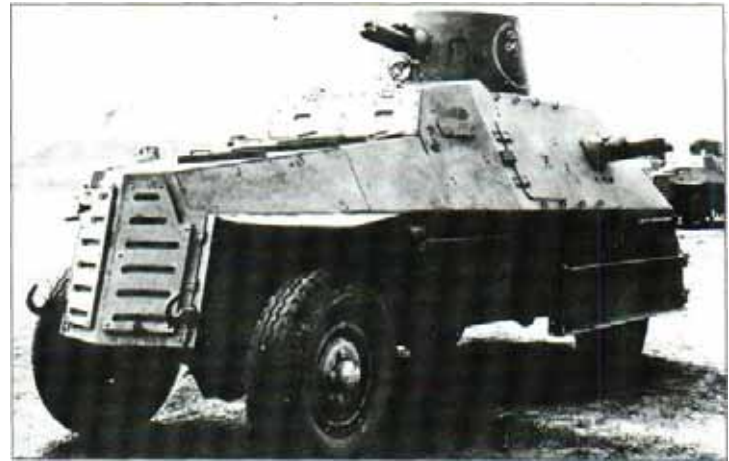
This official photograph shows a Marmon Herrington MkII armoured car in its original form with a Vickers 7.7-mm (0.303-in) machine-gun in the turret and another in a side-mounted mantlet. This latter weapon position was soon discarded and extra weapon positions were provided around the open turret.
