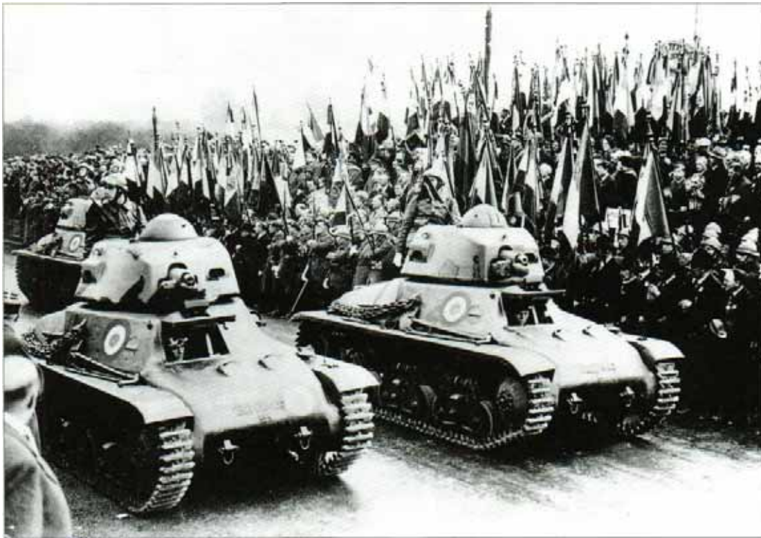
French mechanized units parading with their Hotchkiss H35 tanks. A small, lightly armed vehicle with a crew of two, it saw service with the French in both cavalry and infantry-support roles.
