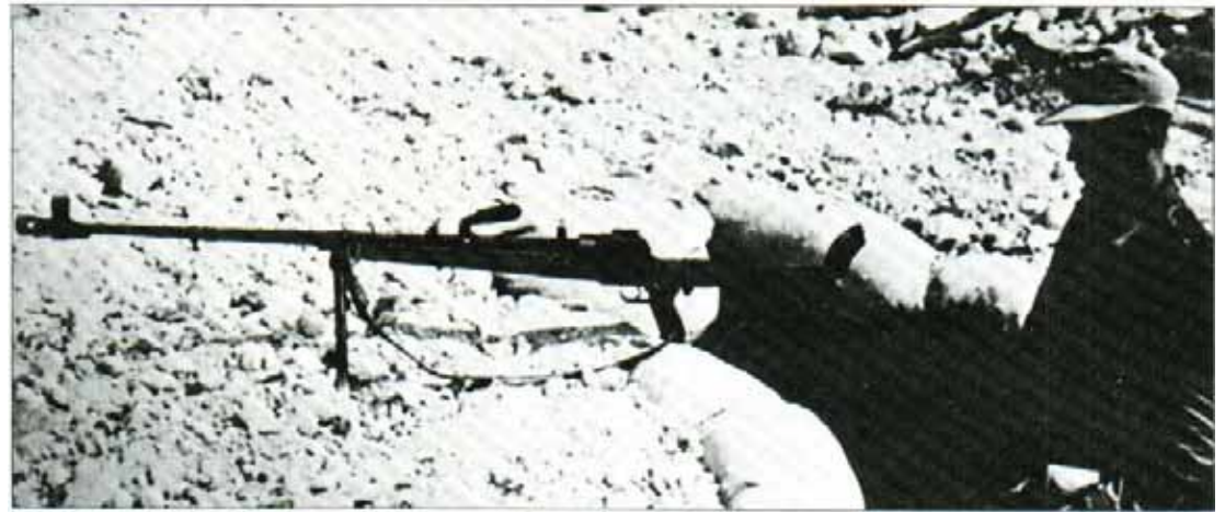
An Africa Korps soldier is seen with a 7.92-mm (0.312-in) Panzerbüchse 39. This was a single-shot rifle that fired tungsten-cored projectiles. The projectile could penetrate 25 mm (0.5-in) of armour at 300 m (328 yards), making it unable to tackle any but the lightest tanks after 1940.
