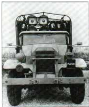
Above: This Canadian-built Ford 3-ton truck is carrying a curious cargo of lighting equipment. Canadian Fords were also produced in Australia, the Ford subsidiary plant in Victoria State re-assembling vehicles for use in the Pacific theatre.
