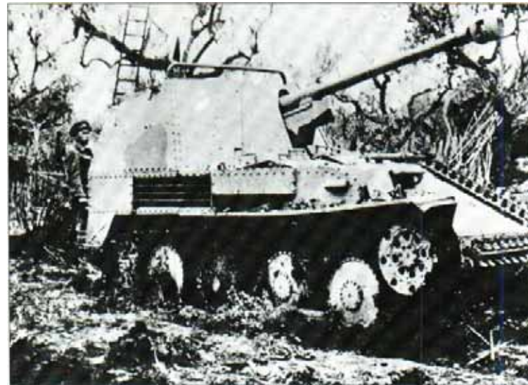
The later Marder IIIs had their main gun position moved to the rear of the chassis and the engine to the front. This provided a better-balanced and
