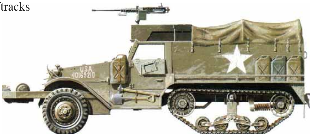
Above: The American M3 halftrack was such a widely used vehicle that it became a virtual trademark of the US Army and other Allied forces, including the Red Army. This M3 is complete with the canvas tilt, a forward-mounted winch and the 'pulpit' machine-gun mounting, here with a 0.50-in (12.7-mm) Browning.
