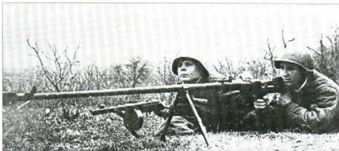
The Soviet 14.5-mm (0.57-in) PTRD 1941 anti-tank rifle has had a round loaded into the breech with the loader's left hand; a subsequent tap on the firer's helmet would then indicate that the rifle is ready to fire.
