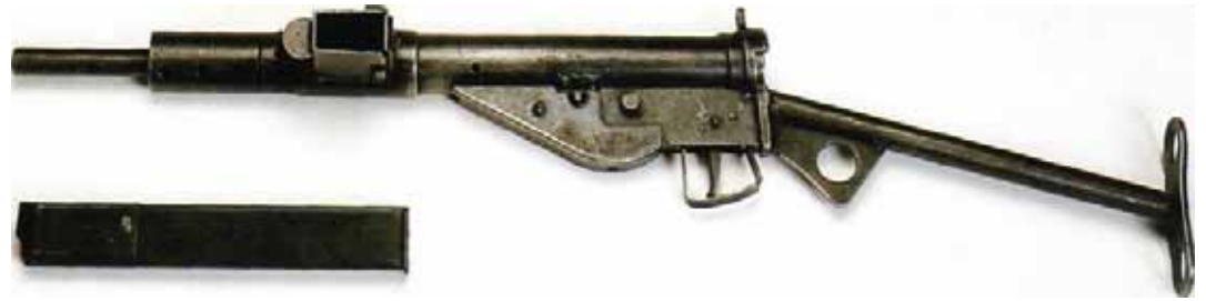
Above: The Sten Mk II was one of the most widely-used of all the Allied sub-machine guns. It looked crude but it worked, it could be stripped down for easy concealment, and it was available in quantity.
