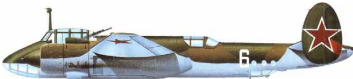
The Tupolev Tu-2S carried two wing root cannon and three machine-guns mounted in the rear cockpit and the dorsal and ventral positions.
