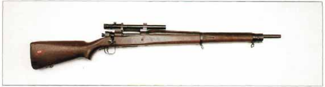
Above: A Mauser patterned rifle, the M1903 Springfield proved a fine weapon, serving into the Korean war. The sniper version had a Weaver telescopic sight, and the conventional 'iron' sights have been removed en tirely.
