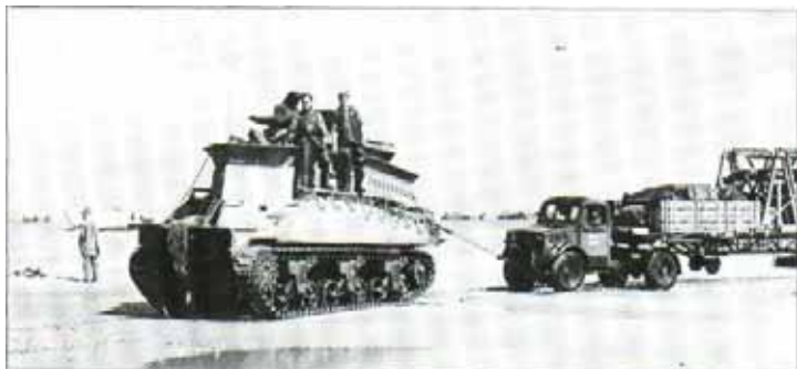
The Sherman BARV (Beach Armoured Recovery Vehicle) was developed during 1943 to tow bogged-down vehicles from deep water during amphibious operations. It was a tractor device only, and the crew usually included a trained diver to secure towing cables to stranded vehicles for towing.
